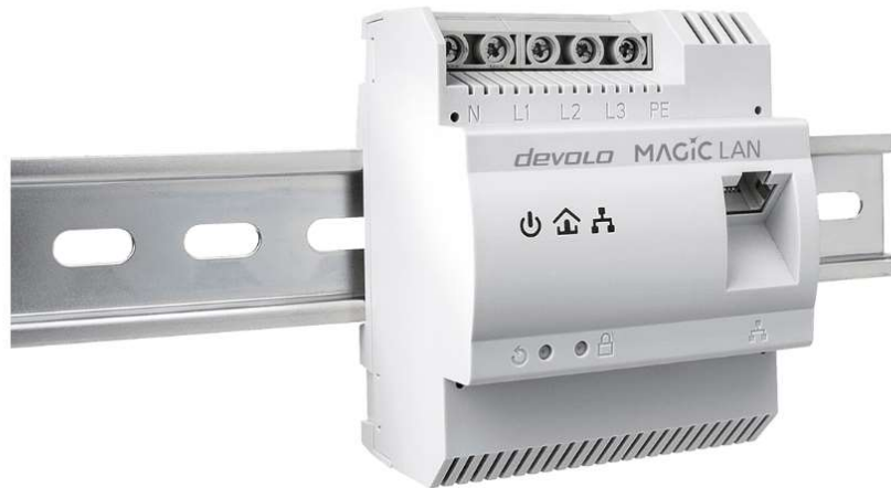
Figure 19 devolo DIN-rail adapter, which can utilize 5 wires for the protective earth conductor, the neutral conductor and three phase conductors of a three-phase system. Please note that all three phases are linked by phase coupling capacitors.
