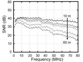
(b) SNR at RX, simplex POF (10 m steps, 40 m not done) Figure 5: Characterization of G.hn PTP POF links
