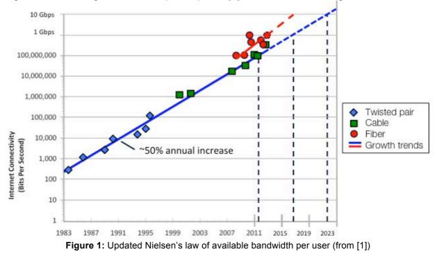
The 50% annual growth in bandwidth offerings has not slowed down for the past 30 years, and global IP traffic has increased eightfold over the past 5 years and will increase nearly fourfold over the next 5 years [2]. Interestingly, the FTTH operators are pushing bandwidth to the home at an even higher rate. It can be expected that 1 Gb/s to the user premises is a commodity in 2015 while at 2017 we could see rates up to 10 Gb/s appearing for the high-end users.
