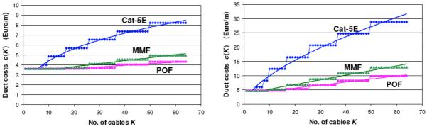
Figure 3: Costs of installed ducts; on-the-wall mounted (I.) and buried (r.) (from [9])
