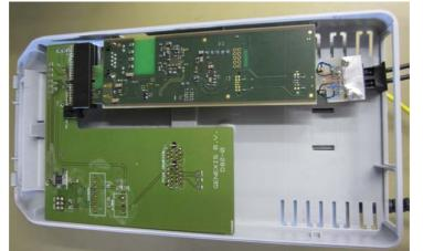
(b) Pluggable module integrated in a Genexis Hybrid FTTH gateway **Figure 2:** omniPOF<sup>™</sup> implementation of POF FITH G.hn
