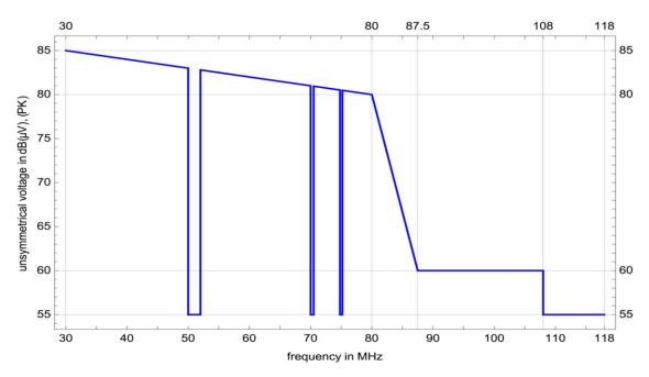
85 dB $\mu$ V<sub>(PK)(unsym)</sub> $\cong$  -81 dBm/Hz<sub>(RMS)(sym)</sub><sup>(\*)</sup>
